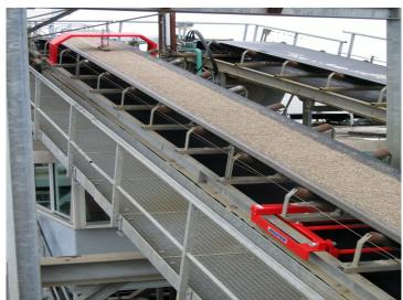
The industrial weighing terminal **IT8000E BELT** captures continuously the quantity of bulk material conveyed over a beltweigher for both, batching and receiving operations.
