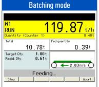
Display of flow rate (large characters) and quantities. Graphic display of operational and process status.
